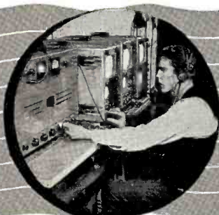
6. REMOTE PICKUP EQUIPMENT — RCA engineers built the first television equipment for field pickups—and the first such equipment (shown here) for use with the "orthicon" camera.
